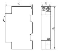
Overvoltage trip release for motor circuit breaker is used to trip the circuit breaker in case of dip or power failure. Installation on the side of the switch.
