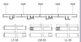
Shade type: matt Enclosure material: aluminum alloy Connection type: Self-clamping block Range of sections of wires used [mm²]: 1,5÷2,5 Lamp-heating time [s]: ≤1 Lamp-ignition time [s]: ≤0,5 IP class: 20
