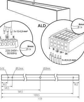
Enclosure material: aluminum alloy Connection type: Self-clamping block
