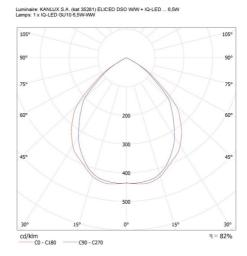
KANLUX S.A. (kat 35281) ELICEO DSO W/W + IQ-LED ... 6,5WS3 / LDC (Polar) Luminaire: KANLUX S.A. (kat 35281) ELICEO DSO W/W + IQ-LED ... 6,5WS3 Lamps: 1 x IQ-LED GUI 0 5,5WS3-WW
