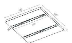
Luminous-flux-retention factor at the end of rated service life : L90B10 Number of on/off cycles: ≥30000 Lighting angle [°]: 50 Luminous efficiency of the lamp [lm/W]: 129 Ambient temperature range to which the product can be exposed: 5÷25 Shade type: louvre Connection type: Self-clamping block Range of sections of wires used [mm²]: 1,5÷2,5 Rodzaj soczewki [°]: 50 IP class: 20 UGR: ≤16
