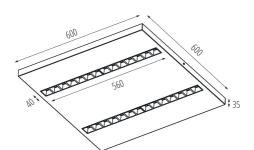
Luminous-flux-retention factor at the end of rated service life : L90B10 Number of on/off cycles: ≥30000 Lighting angle [°]: 50 Luminous efficiency of the lamp [lm/W]: 139 Ambient temperature range to which the product can be exposed: 5÷25 Shade type: louvre Connection type: Self-clamping block Range of sections of wires used [mm²]: 1,5÷2,5 Rodzaj soczewki [°]: 50 IP class: 20 UGR: ≤15
