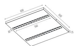
Luminous-flux-retention factor at the end of rated service life : L90B10 Number of on/off cycles: ≥30000 Lighting angle [°]: 80 Luminous efficiency of the lamp [lm/W]: 129 Ambient temperature range to which the product can be exposed: 5÷25 Shade type: louvre Connection type: Self-clamping block Range of sections of wires used [mm²]: 1,5÷2,5 Rodzaj soczewki [°]: 80 IP class: 20 UGR: ≤16
