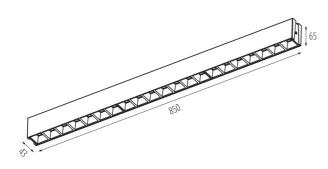
Connection type: Self-clamping block Range of sections of wires used [mm<sup>2</sup>]: 1,5÷2,5 IP class: 20 UGR: <17
