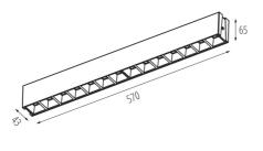
Enclosure material: steel, plastic Connection type: Self-clamping block Range of sections of wires used [mm<sup>2</sup>]: 1,5÷2,5 IP class: 20 UGR: <18
