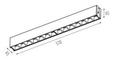
Enclosure material: steel, plastic Connection type: Self-clamping block Range of sections of wires used [mm<sup>2</sup>]: 0,5÷2,5 IP class: 20 UGR: <18
