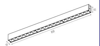
**Enclosure material**: steel, plastic **Connection type**: Self-clamping block
