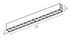
Enclosure material: steel, plastic Connection type: Self-clamping block Range of sections of wires used [mm<sup>2</sup>]: 0,5÷2,5 IP class: 20 UGR: <17
