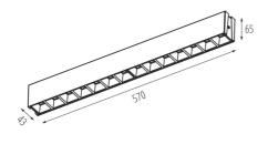
**Enclosure material**: steel, plastic **Connection type**: Self-clamping block
