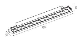
Enclosure material: steel, plastic Connection type: Self-clamping block Range of sections of wires used [mm<sup>2</sup>]: 1,5÷2,5 IP class: 20 UGR: <17
