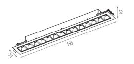
Enclosure material: steel, plastic Connection type: Self-clamping block Range of sections of wires used [mm<sup>2</sup>]: 1,5÷2,5 IP class: 20 UGR: <16
