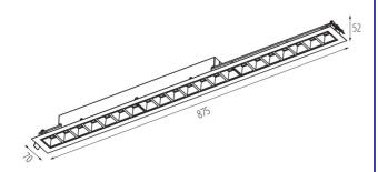
Connection type: Self-clamping block Range of sections of wires used [mm<sup>2</sup>]: 1,5÷2,5 IP class: 20 UGR: <17
