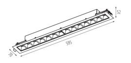
Connection type: Self-clamping block Range of sections of wires used [mm<sup>2</sup>]: 1,5÷2,5 IP class: 20 UGR: <17
