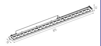
Connection type: Self-clamping block Range of sections of wires used [mm<sup>2</sup>]: 1,5÷2,5 IP class: 20 UGR: <16
