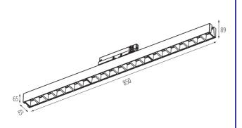
Enclosure material: steel, plastic IP class: 20 UGR: <17
