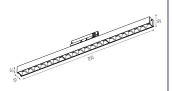
Enclosure material: steel, plastic IP class: 20 UGR: <15
