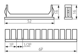
End cap for switchboards used to mask unused spaces on the rail. The set contains two 1P (17.5mm) end caps and eight 0.5P (8.75mm) end caps.
