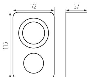
Kanlux STER TS-MF is an adapter of an extension socket with a 24-hour mechanical programmer. It makes it possible to programme turning on and turning off operations for connected devices at pre-set time.
