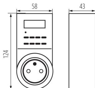
Kanlux CYBER is an adapter of an extension socket with a 24-hour digital programmer. It makes it possible to programme turning on and turning off operations for connected devices at pre-set time.
