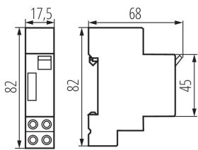
Staircase lighting timer is used to keep lighting on for a set period of time; adjustable time range from 1min to 7min, the accuracy of the programmed time setting is 0.5min.
