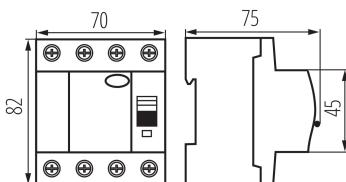
Residual current circuit breaker: is used for additional protection against electric shock, designed for work in sinusoidal alternating current circuits (AC type) and sinusoidal alternating and pulsating current with DC component (A type).
