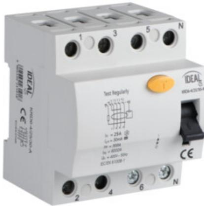
Residual current circuit breaker: is used for additional protection against electric shock, designed for work in sinusoidal alternating current circuits (AC type) and sinusoidal alternating and pulsating current with DC component (A type).
