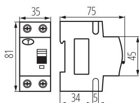
Residual current device with overcurrent protection is used to protect against overloads and short circuits in installations and devices, as well as to protect against electric shock.
