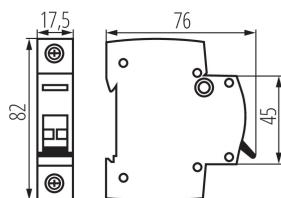
Switch disconnector is used to disconnect circuits loaded with rated current.
