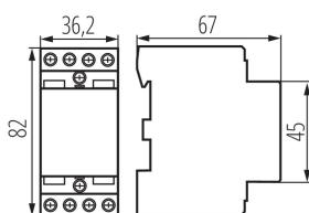
Contactor is used for automatic activation of electricity receivers. Categories of use AC7a, AC7b.
