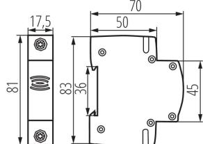
Electric bell is used for sound signalling without the need to use a bell transformer. Power supply from a 230VAC power grid.
