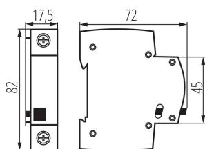
Space reserve module for switchboard, installation on a TH35 rail, width of one module (17.5mm).
