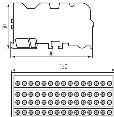
Terminal block is used for power distribution, it is adapted to cable lugs.
