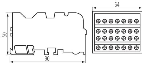
Terminal block is used for power distribution, it is adapted to cable lugs.
