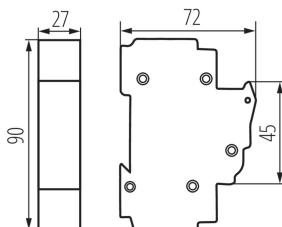
Switch disconnector with a KSF fuse is an apparatus enabling replacement of the fuse element protecting electrical installations with D02 system fuses.
