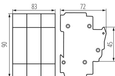
Switch disconnector with a KSF fuse is an apparatus enabling replacement of the fuse element protecting electrical installations with D02 system fuses.
