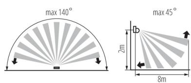
ALER MINI-W sensor is a small infrared sensor with attractive and minimalistic design. The horizontal angle of the sensor work comes to 140°, and vertical 45°, and thanks to easy mechanical adjustment (vertical 45°, level 90°) it can be adapted to your needs. Owing to the high class of tightness (IP44), this sensor can be mounted in places directly exposed to weather conditions.
