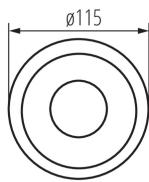
Kanlux ZONA FLAT is a motion detector with maximum motion detection range of 8m. In turn, its maximum horizontal angle of work comes to 360 degrees. In the ZONA sensor, you can adjust the time of lighting from 10s to 15min as well as set the surrounding light intensity level at which the device will work.
