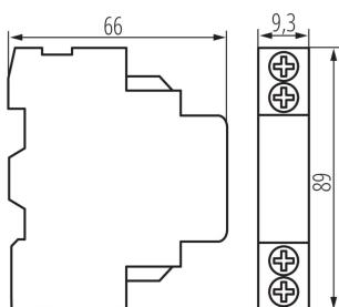
Auxiliary contact for the switch, mounted on the side of the switch. 1NO+1NC contacts.
