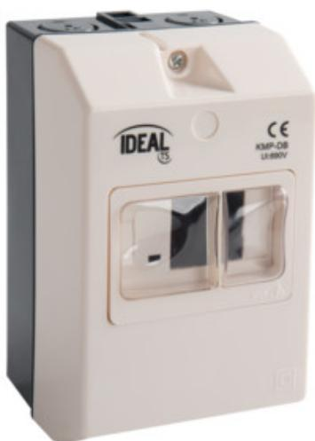
Housing for motor circuit breakers, tightness class IP65. The housing fits one motor circuit breaker, one 17.5mm wide module and one 8.75mm wide module. The housing has transparent windows used for operating the power switch buttons.
