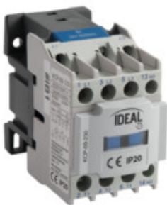
Power contactors are designed to connect AC circuits in AC3 utilisation category. Current range of the offer up to 32A, supply voltage 24VAC or 230VAC. As a standard, contactors have a 1NO auxiliary contact.
