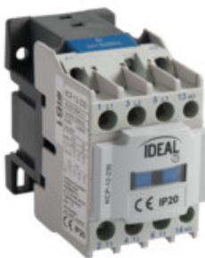
Power contactors are designed to connect AC circuits in AC3 utilisation category. Current range of the offer up to 32A, supply voltage 24VAC or 230VAC. As a standard, contactors have a 1NO auxiliary contact.
