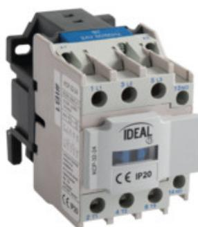
Power contactors are designed to connect AC circuits in AC3 utilisation category. Current range of the offer up to 32A, supply voltage 24VAC or 230VAC. As a standard, contactors have a 1NO auxiliary contact.
