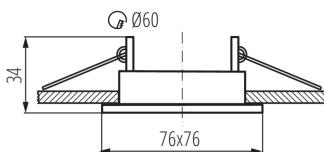
Kanlux ALOR is a family of downlights in the most popular colors; black and white, with a matte finish. Downlight do not have a ceramic lamp holder in the set. We can use the lamp holder that will fit the GU10 or Gx5.3 base, which will allow us to use light sources adapted to the prepared installation.
