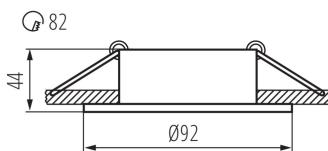
Kanlux IVRI is a decorative ring made of aluminium. Kanlux IVRI is expressive in its shape and adjustment of the direction of light - light source comes to 30 degrees.
