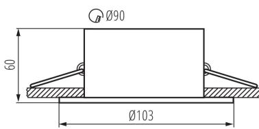
Kanlux APRILA is a family of white decorative rings made of aluminium. Kanlux APRILA has a streamlined shape and can be adjusted in terms of the angle of light within the range of 20 degrees. The JDR or MR-16 frame can be used for the holders, which will allow us to use light sources adapted to a prepared installation.
