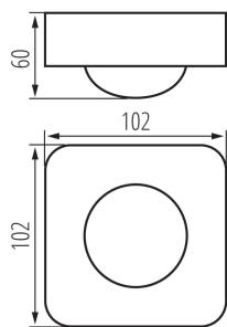
Kanlux SENTO is an electronic sensor for movement detection. Its exceptionality lies in the fact that as many as three infrared detectors are installed in one sensor. This guarantees an unprecedented sensitivity and allows you to capture even the slightest movement. Kanlux SENTO, due to its unusual features, is referred to as a presence detector.
