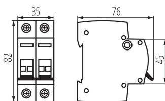
Switch disconnector is used to disconnect circuits loaded with rated current.
