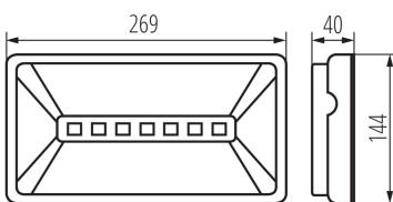
Emergency or anti-panic lighting is used in open space rooms to prevent panic. It allows you to reach a place where you can see the marked escape route as well as for the illumination of the escape route itself, depending on the prism used in the fixture.
