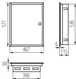
Metal Consumer Units with DIN rails for modular installation are manufactured at the Kanlux Factory. They are designed for public and office buildings. Their scope allows you to carry out installations also in areas such as extensive residential installations.
