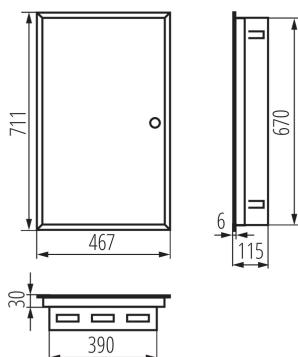
Metal Consumer Units with DIN rails for modular installation are manufactured at the Kanlux Factory. They are designed for public and office buildings. Their scope allows you to carry out installations also in areas such as extensive residential installations.
